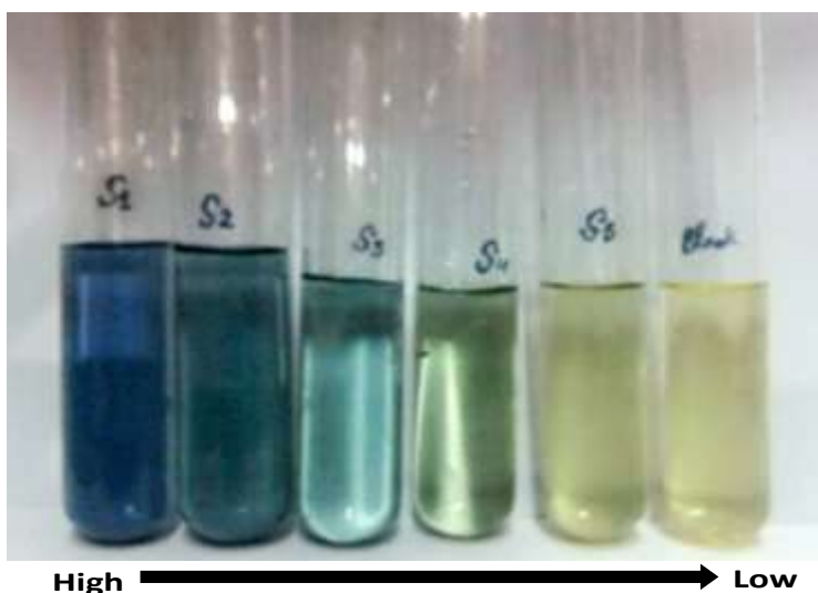
Figure 2. Standard solutions showing gradual decrease in amylose concentration
