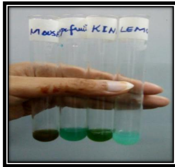
Fig. 2: Positive Benedict's test with citrus juices showing presence of reducing sugar in fresh juices except in tetra pack juice.
